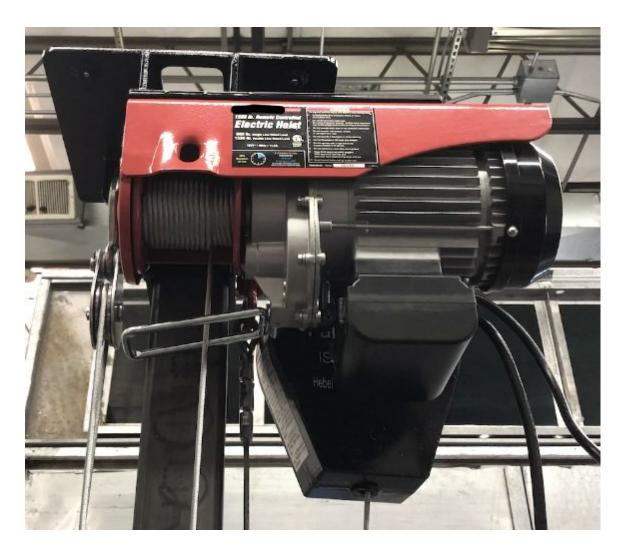
10.5. Here is the Hoist, Hoist Head, SRL and pulleys mounted on top of the Column, looking from the back side.
