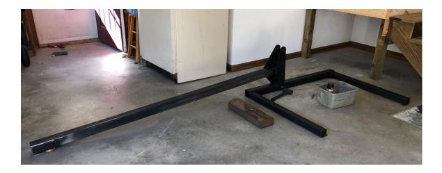
16.5. Line up the bottom hole in the flange with the end hole of the four (4) hole pattern in the Base. In the case of the illustration below, the BOTTOM hole of the flange must be aligned with the LEFT most hole in the Base.
