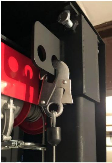
24.4. Rotate the SRL body so that it will not interfere with the Limit Switch. Make sure the SRL strap is not twisted and then attach the SRL's carabiner through the outer hole.
