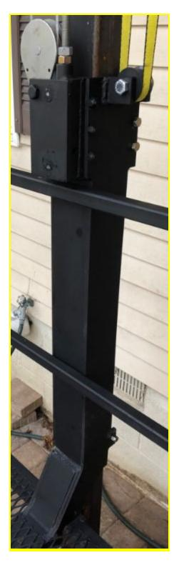
7.9. **Column** - Supports the Hoist and the Safety Retractable Lanyard (SRL). (Note - the photo below is without the Safety Guard and also shows an obsolete Hoist Cover)
