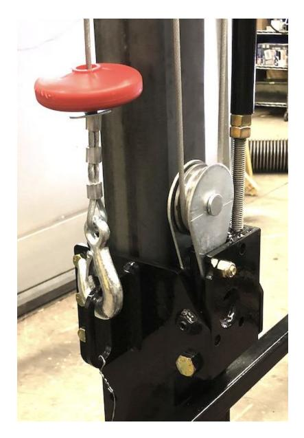
10.8. Here is how the hoist cables and pulleys should be configured, from the left/front side.
