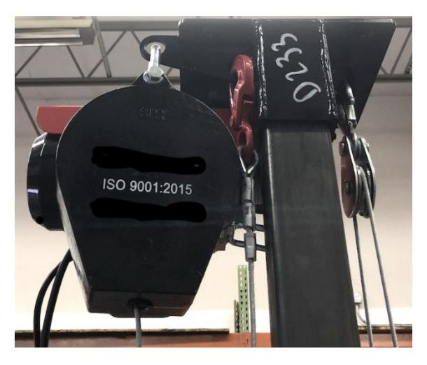
10.6. Here is the Hoist, Hoist Head, SRL and pulleys mounted on top of the Column, looking from the left side.
