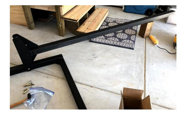
17.3. Carefully attach the Hoist Head by sliding it on the end of the Column. The flat side of the Hoist Head goes to the back of the Column. The cable needs to run down the Platform side of the Column.
