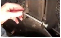
19.13. Tighten the lock-nut until it will not come off the bolt and no more. **The bolt should be able to be spun freely by hand.**
