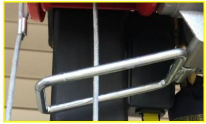
7.17. **Limit Switch Actuator** - This customer adjustable assembly triggers the Limit Switch to stop the Platform at the Landing height. The photo below shows the various parts of this assembly - the adjustable metal rod, the black EMT/PVC pipe with the trigger, and the grommet (with slot) that protects the cable from wear. Note: This approach has been replaced by the Upper Limit Switch (see below).
