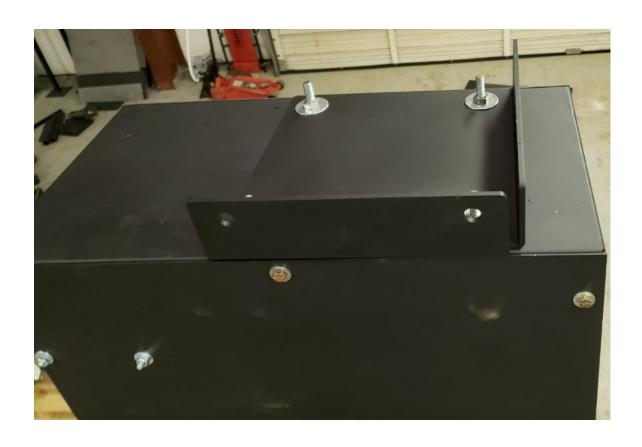
7.6. **Brace Kit** - Bracing steadies the Column and eliminates any Platform"bounce". This feature is optional on lifts of 4' station height or less and is required on medium height lifts between 4' and 6'. Above 6' a Bracket Cap approach is required. Below is a photo of our Brace Kit that connects the top of the Column to a nearby wall.
