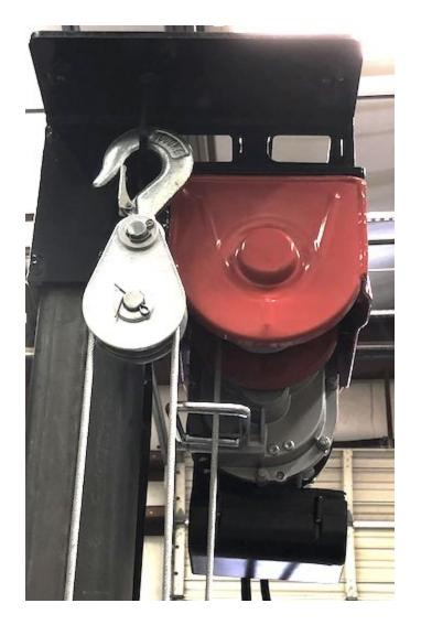
10.7. Here is the Hoist Hook, Pulley Block, Threaded Rod (with nuts) and stop rod. looking from the left/front side.
