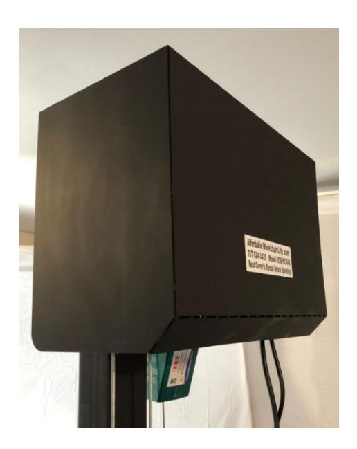
7.14. **Hoist Head** - The Hoist attaches to the Hoist Head. The Hoist Head mounts on top of the Column. In the photo below the Hoist Head is the black metal part.
