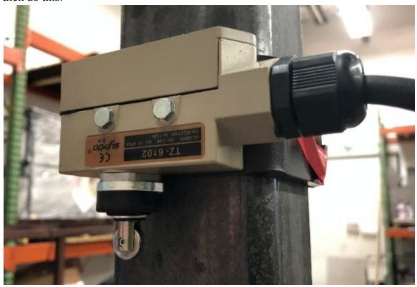
19.20.1. Mount the shiny sheet metal Spring Actuator portion of the Upper Limit Switch to the back of the Collar using the existing bolts found there:
